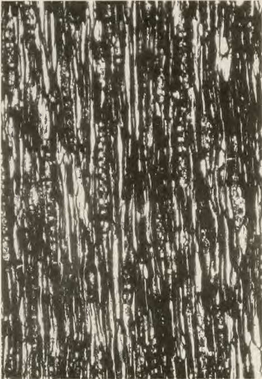
Fig. 18. Tangential longitudinal section showing distorted rays. x 125.
